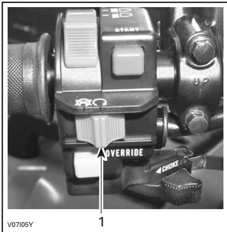
TYPICAL 1. Engine stop switch
