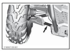
Strap the rear tires by using tire towing straps.
