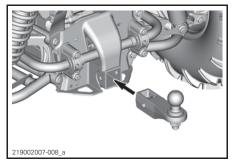
Insert the pin through the draw bar and receiver hitch.
