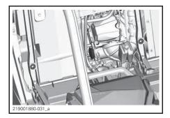
Remove oil filter cover. Remove oil filter.
