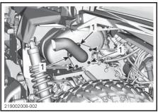
1. Tail pipe retaining screws
