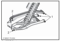
1. M12 fasteners 2. M10 fasteners
