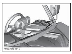
Refer to ACCESSING MAINTENANCE COMPONENTS and remove the seats backrest.
