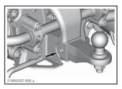
Secure the pin by folding the lock.
