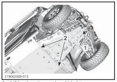
Lifting location under skid plate
