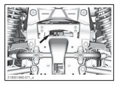
Under the vehicle, place a drain pan underneath the oil drain plug area.
