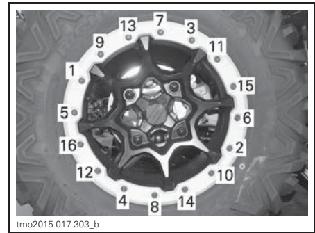
TYPICAL - TIGHTENING SEQUENCE
