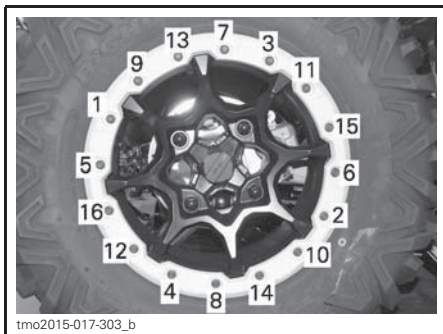
TYPICAL - TIGHTENING SEQUENCE
