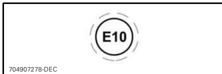
LOCATED NEAR GAS CAP
