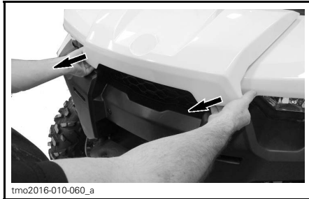
PULLING ON FRONT SERVICE COVER EDGE.
