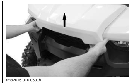
LIFTING FRONT SERVICE COVER EDGE.
