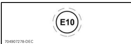
LOCATED NEAR GAS CAP
