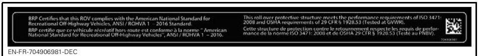
LOCATED ON TOP LH BAR OF CAGE FACING THE INSIDE OF VEHICLE
