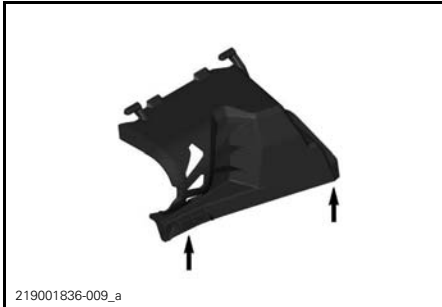
LIFTING REAR OF SERVICE COVER
