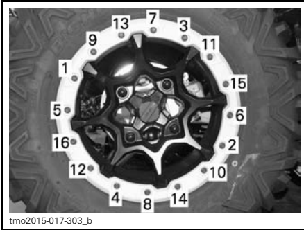
TYPICAL - TIGHTENING SEQUENCE
