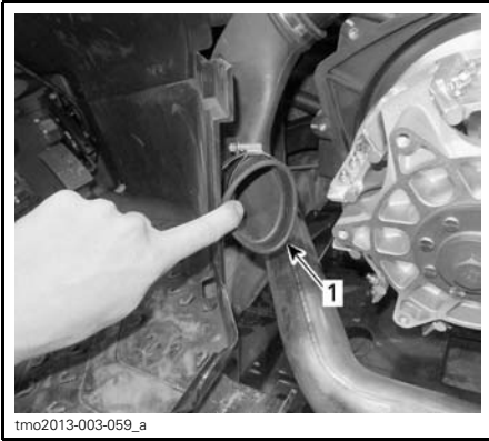
TYPICAL 1. Inside CVT outlet hose
