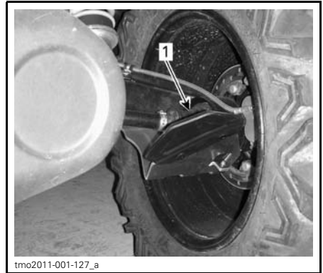
REAR OF VEHICLE 1. Outer drive shaft boot
