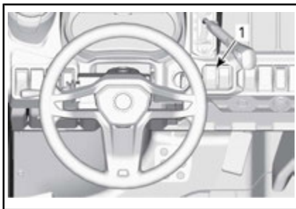
1. Bryteren for tohjuls/firehjuls drift
