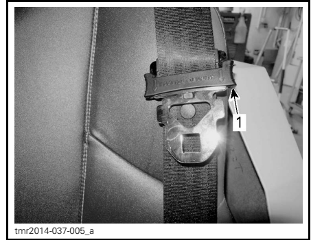
TYPICAL - LOCKED POSITION
