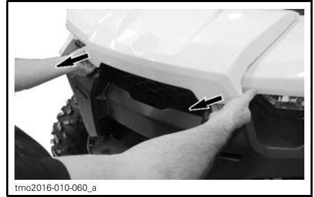
tmo2016-010-060_a PULLING ON FRONT SERVICE COVER EDGE.
