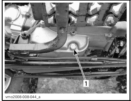
LH SIDE OF ENGINE 1. Drain plug
