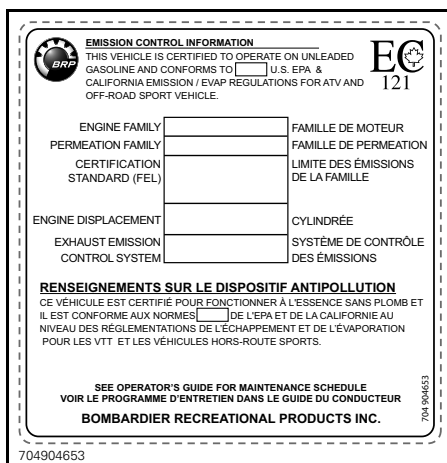
TYPICAL LABEL 2 - BEHIND SEAT: VEHICLES COMPLIANT TO US EPA STANDARDS OR EQUIVALENT
