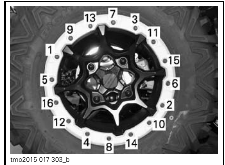
TYPICAL - TIGHTENING SEQUENCE
