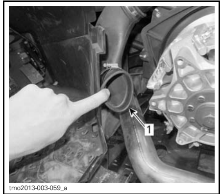
TYPICAL 1. Inside CVT outlet hose
