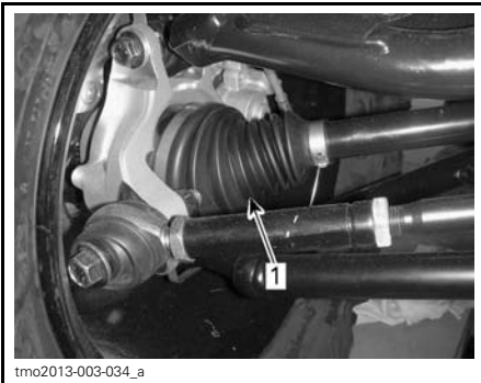
REAR OF VEHICLE 1. Outer drive shaft boot
