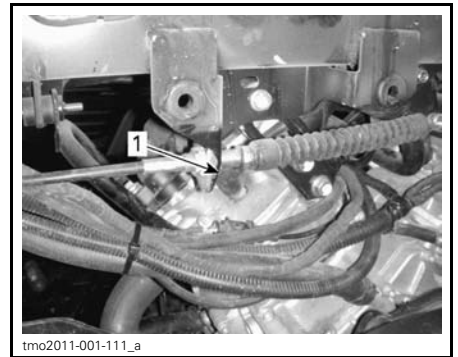
LH SIDE — FRONT CYLINDER 1. Spark plug
