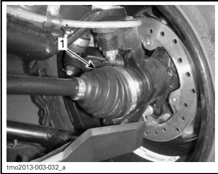
FRONT OF VEHICLE 1. Outer drive shaft boot
