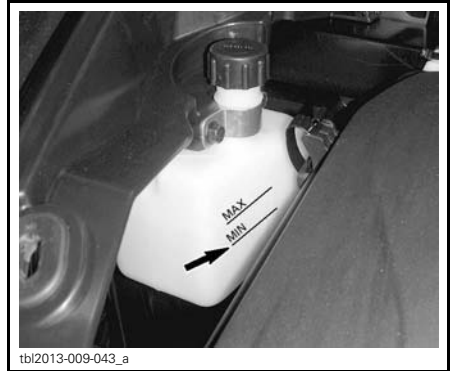
TYPICAL - COOLANT EXPANSION TANK
