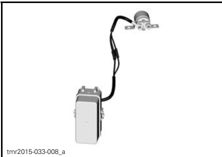
FUSIBLE LINK CONNECTED TO FUSE BOX
