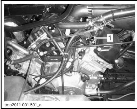
1. Front cylinder bleed screw
