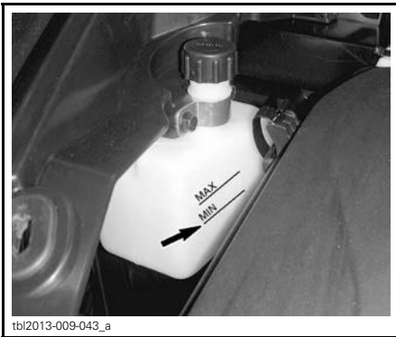
COOLANT EXPANSION TANK
