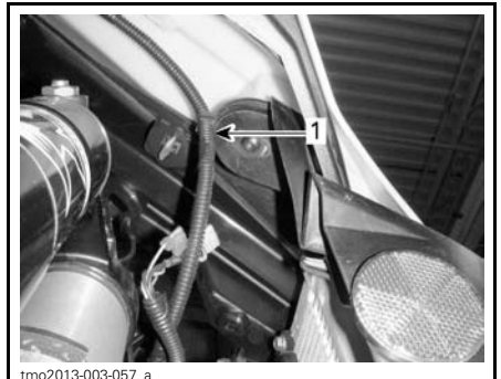
LOCATED BEHIND RH SIDE OF RADIATOR COVER 1. Electrical cable
