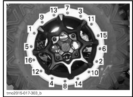
TYPICAL - TIGHTENING SEQUENCE
