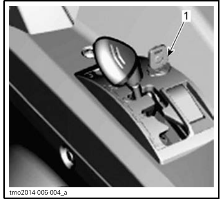
TYPICAL - SHIFT LEVER CAN BE LOCKED IN PARKED POSITION 1. Shift lever locking key
