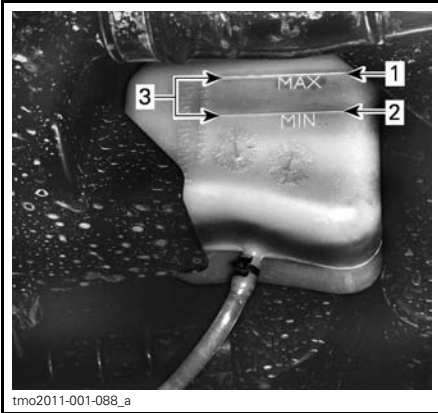
COOLANT EXPANSION TANK
