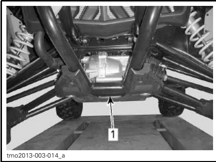
FRONT OF VEHICLE 1. Hydraulic jack position
