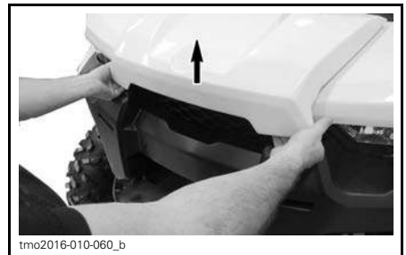
LIFTING FRONT SERVICE COVER EDGE.
