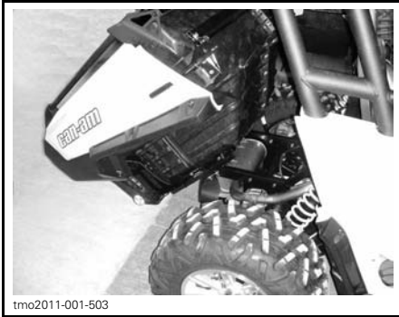
tmo2011-001-503 FRONT SECTION OF INCLINED CARGO BOX FREE OF ANY OBJECTS
