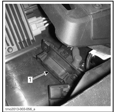
1. Auxiliary fuse box
