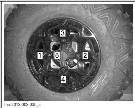
TIGHTENING SEQUENCE - TYPICAL
