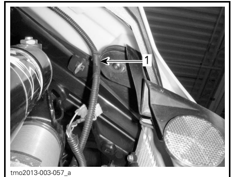
LOCATED BEHIND RH SIDE OF RADIATOR COVER
