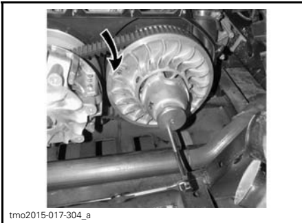
1. Lowest portion of cogs even with external surface of drive belt
