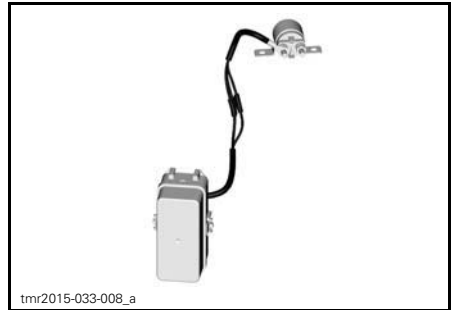
FUSIBLE LINK CONNECTED TO FUSE BOX
