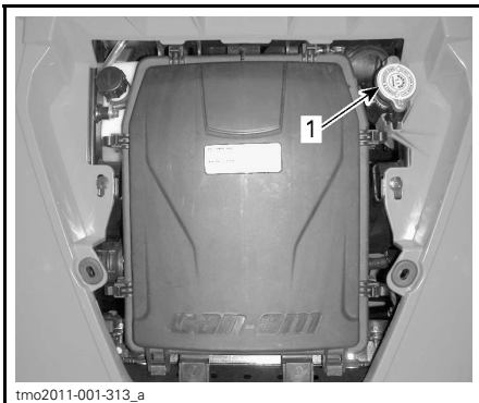
1. Radiator pressure cap
