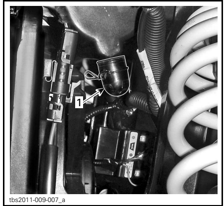
1. Remove drain plug to expel water
