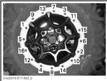
TYPICAL - TIGHTENING SEQUENCE
