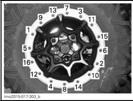
TYPICAL - TIGHTENING SEQUENCE
