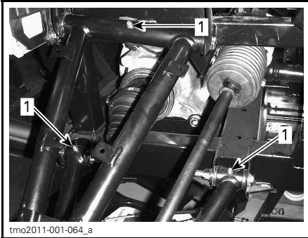
FRONT SUSPENSION - TYPICAL 1. Grease fittings
