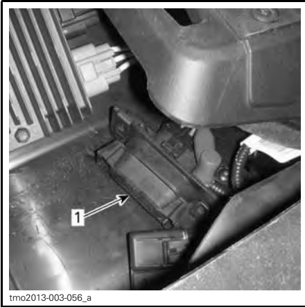
1. Auxiliary fuse box
