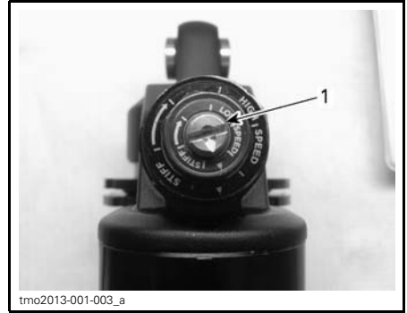
TYPICAL - XT-P MODEL 1. Low speed compression adjuster
