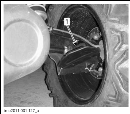
REAR OF VEHICLE 1. Outer drive shaft boot
