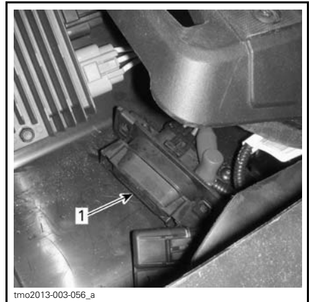
1. Auxiliary fuse box
