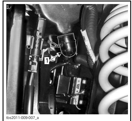
1. Remove drain plug to expel water
