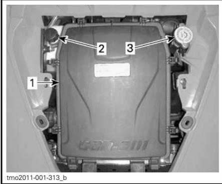
1. Engine air filter housing cover
