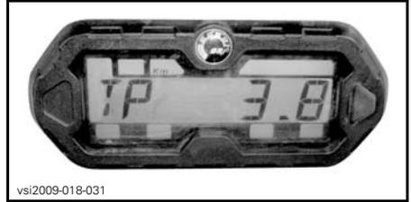
It can be used to establish a fuel tank range or distance between 2 way points for instance.
