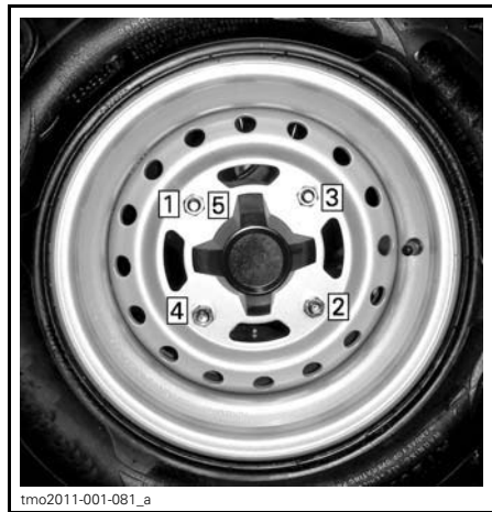
TIGHTENING SEQUENCE
