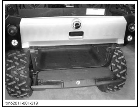
TYPICAL - LOWER SECTION WITH LOWER TAILGATE
