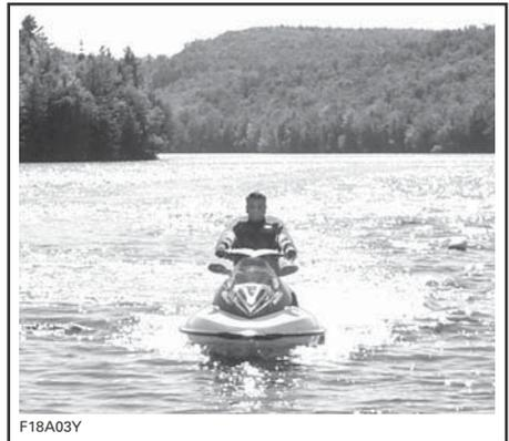
The operator should practice in open waters at various speeds to become familiarized with the stopping distances under different conditions. Stopping using the iBR system in a straight line and in a turn should be practiced exten-
