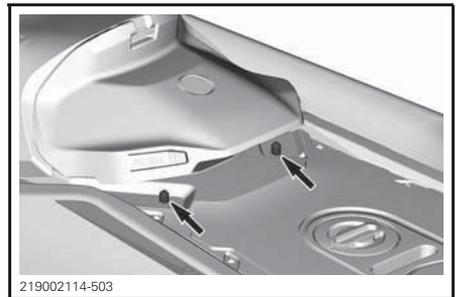
4. Pull up on the the seat back end to ensure it is properly latched.
