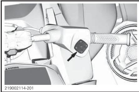
The right controller includes controls to navigate in the multifunction gauge.
