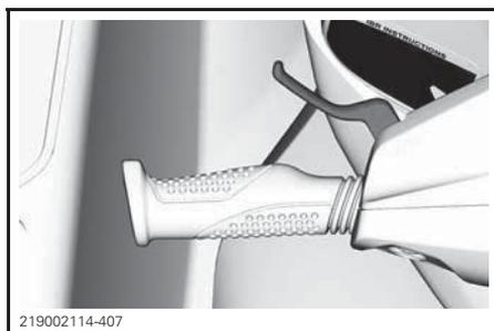
4. When the **iBR OVERRIDE - PRESS MODE BUTTON** message appears in the multifunction gauge, press the MODE button.
