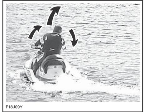
Turning the handlebar pivots the jet pump nozzle which controls the watercraft direction. Turning the handlebar to the right will turn the watercraft to the right and inversely. You need to apply throttle to steer.
