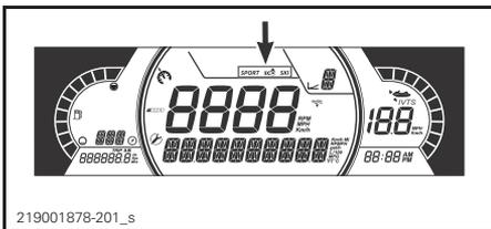
The MODE display indicate the selected alternative mode of operation:
