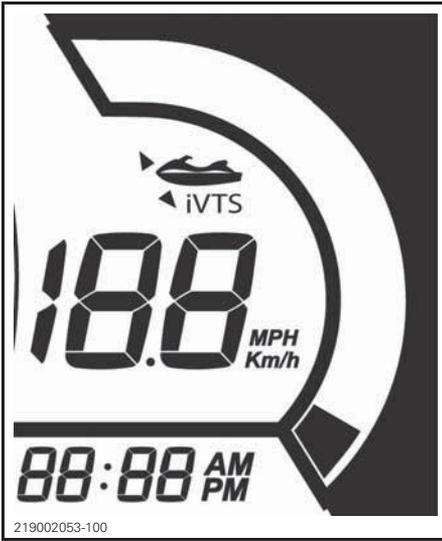
To select the mid trim position, it depends on the actual trim position. Double-click on the VTS UP button if it is positioned below mid trim or double-click on the VTS DOWN button if it is positioned above mid trim.
