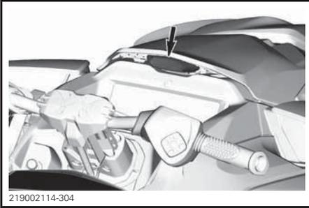
**NOTICE** The maximum load allowable for the front storage compartment is 13 kg (30 lb) evenly distributed.
