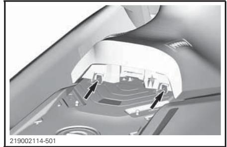
3. Align the seat back end latches with the latch pins and firmly press down on the seat back end to lock it in place.
