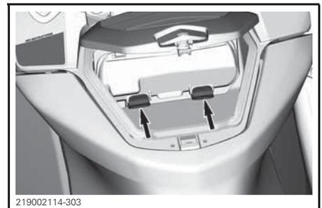
There is a protective foam located inside the watertight compartment to protect a phone from damages. Make sure the smartphone is held in place by
