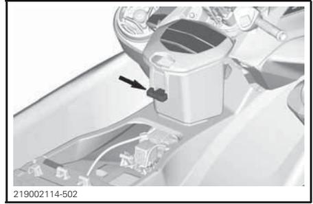
2. Insert the forward part of the seat back end into the retainers.
