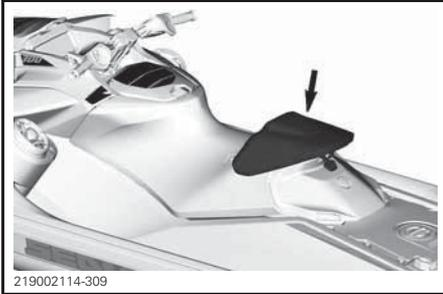
This seat saddle provides a support so that the driver's thighs are properly engaged in the ergolock which has the effect of increasing its efficiency and allow the driver to withstand greater lateral acceleration by transferring force to the pelvis rather than the upper body.
