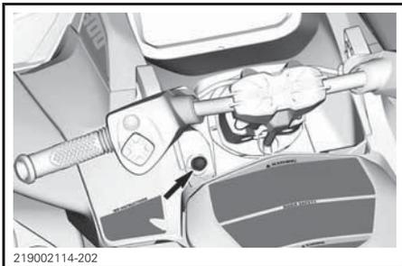
To allow engine starting, the tether cord cap must be securely snapped to the engine cut-off switch.
