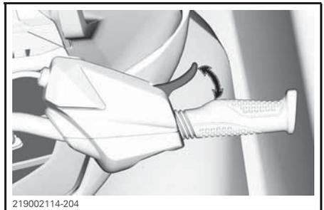
The throttle lever is spring loaded and should return to rest position (idle) when not pressed.
