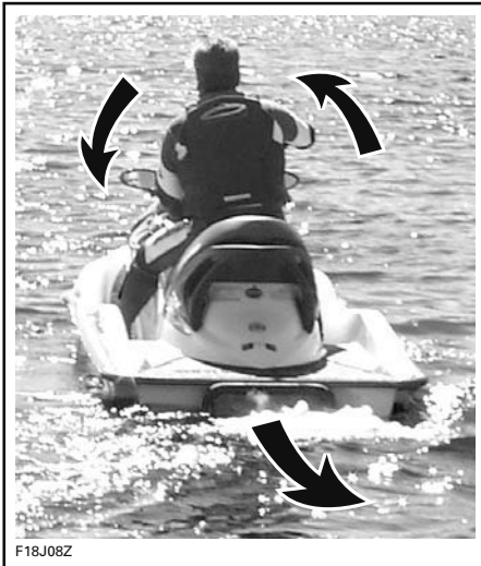
TYPICAL - STEERING DIRECTION REVERSED WHEN BACKING
