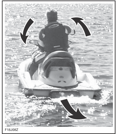
TYPICAL - STEERING DIRECTION REVERSED WHEN BACKING
