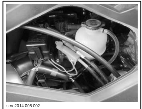
ENGINE COMPARTMENT - LH ACCESS COVER REMOVED
