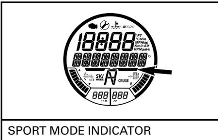
**NOTE:** Sport mode is not the default riding mode. To be active, it must be selected after starting the engine.
