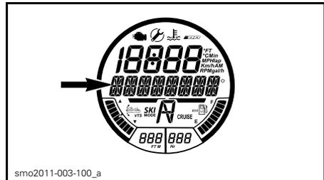
3. Press the UP button until the desired cruise speed is indicated in the numerical display.
