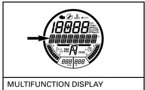
**NOTE:** The default indication in the multifunction display is the compass direction.
