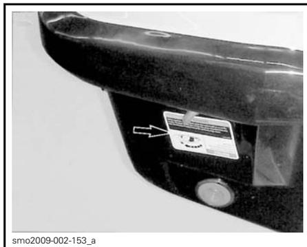
The 4-TEC™ engine features a tip-over protection system (T.O.P.S.™). When the watercraft tips over, the engine is automatically stopped.
