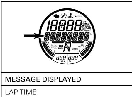
2. Press the SET button to enter the function, the lap timer will be activated and visible in the display.
