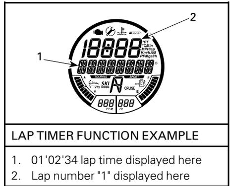
5. To save the last lap and stop the timer, press the MODE button.
