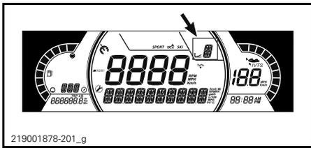
This display the gears position of gear-box:
