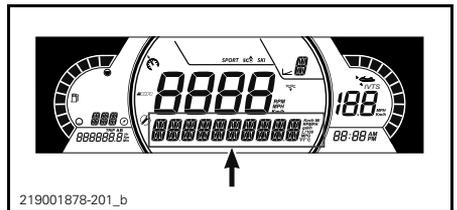
To deactivate the **Launch Control**, press simultaneously both UP/DOWN buttons again.
