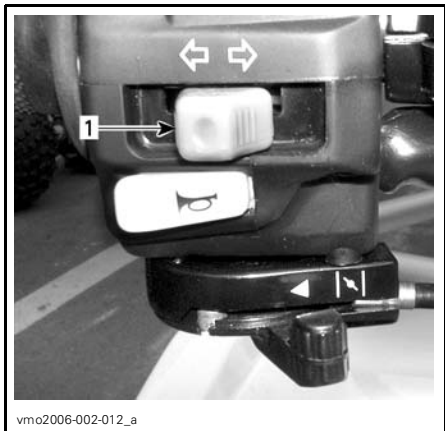
1. Direction indicator switch
