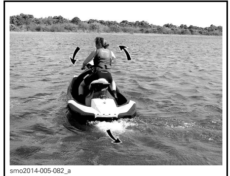
TYPICAL - STEERING DIRECTION REVERSED WHEN BACKING
