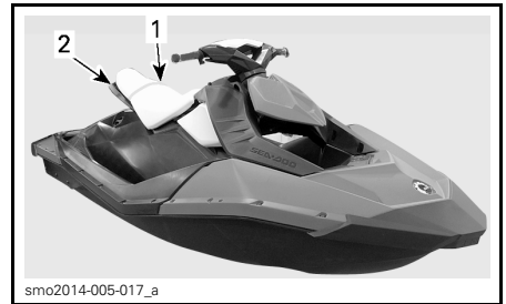
TYPICAL - PASSENGER HANDHOLDS 1. Seat strap 2. Molded grab handle
