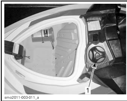
TYPICAL - FUEL TANK CAP LOCATION
