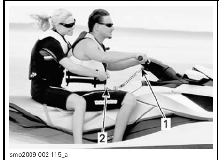
TYPICAL 1. Tether cord cap on the engine cut-off switch 2. Tether cord clip secured to operator's PFD
