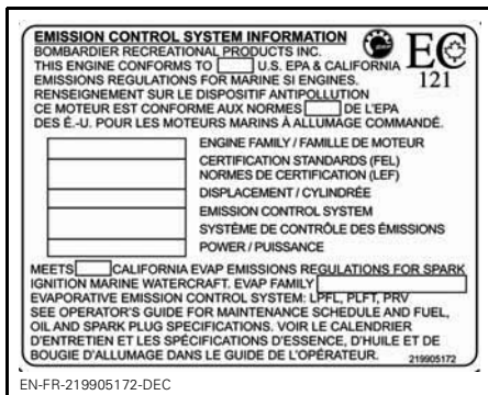
LABEL 2 - APPLICABLE FOR ALL MODELS IN CANADA AND UNITED STATES, APPLICABLE FOR MODELS EVERYWHERE EXCEPT CANADA AND UNITED STATES WHEN EQUIVALENT TO A MODEL CERTIFIED TO US. EPA STANDARDS
