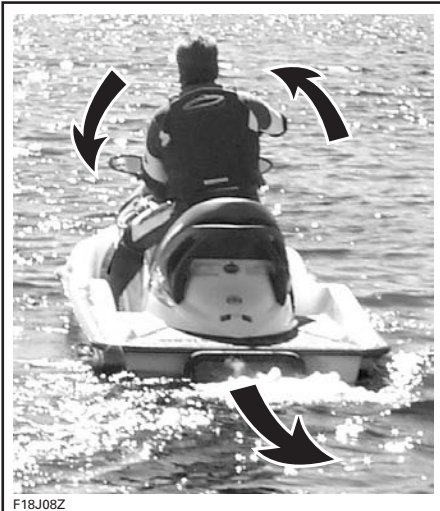
TYPICAL - STEERING DIRECTION REVERSED WHEN BACKING
