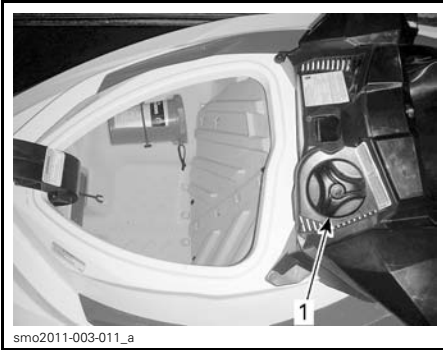
TYPICAL - FUEL TANK CAP LOCATION
