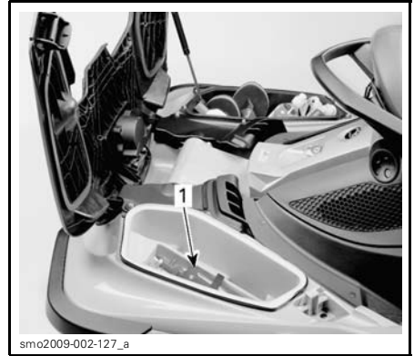
1. Fire extinguisher holder location
