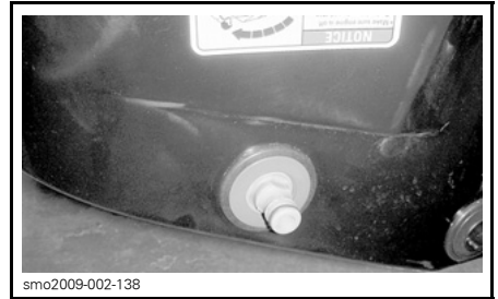
TYPEBILDE – SLANGEOVERGANG FOR HURTIGKOBLING
