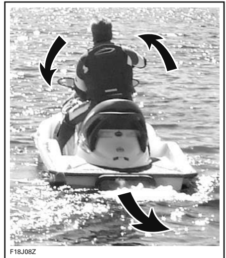
TYPICAL - STEERING DIRECTION REVERSED WHEN BACKING
