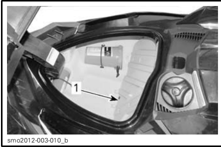
TYPICAL - FRONT STORAGE COMPARTMENT COVER OPENED 1. Access panel
