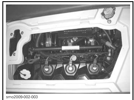
VENTILATION BOX REMOVED
