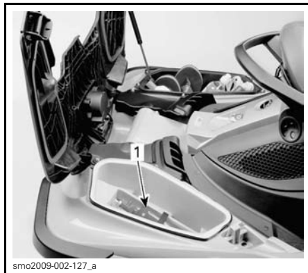
1. Fire extinguisher holder location
