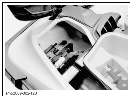
BATTERY AND FUSE ACCESS - RH STORAGE BIN REMOVED
