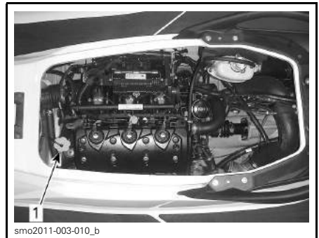
TYPICAL 1. Oil filler cap location
