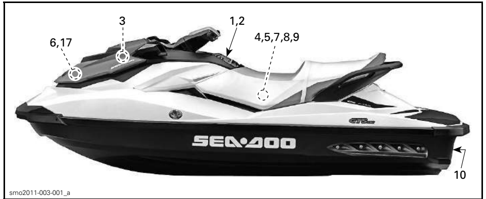
WATERCRAFT SAFETY LABEL LOCATION - GTS MODELS
