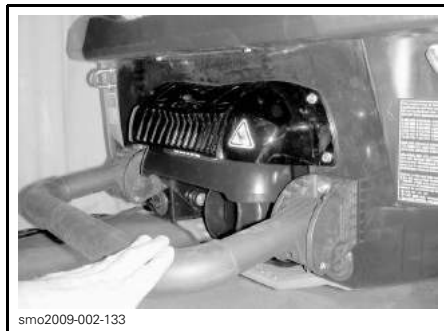
TYPICAL - BOARDING STEP HELD DOWN FOR BOARDING FROM WATER
