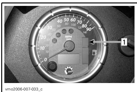
vmo2006-007-033_c 1. Position de la transmission
