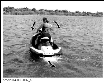
TYPICAL - STEERING DIRECTION REVERSED WHEN BACKING
