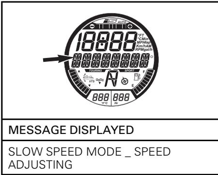
The setting point indication in the digital screen will come back on to indicate the slow speed setting change.
