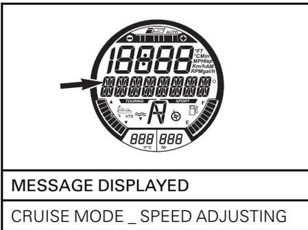
3. Press the UP/DOWN button to adjust speed accordingly.
