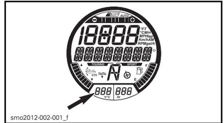
The numerical display may also be selected to display water temperature. See *NUMERICAL DISPLAY* in this section.
