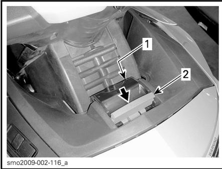
**STEERING COLUMN ADJUSTMENT LATCH NOT SECURED**
