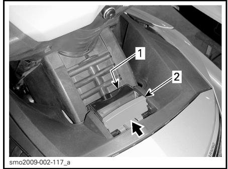
**STEERING COLUMN ADJUSTMENT LATCH PROPERLY SECURED**
