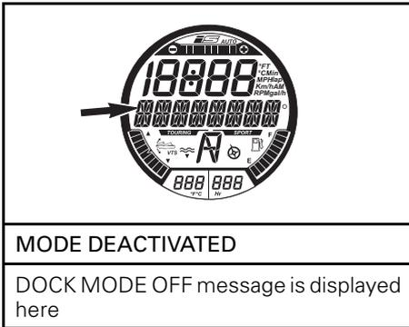
7. Press the SET button, or wait for the function to time out to save the setting and return to main display.
