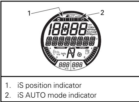
When the suspension system is operating in AUTO mode, the AUTO indicator and all bar segments of the position indicator will be on.
