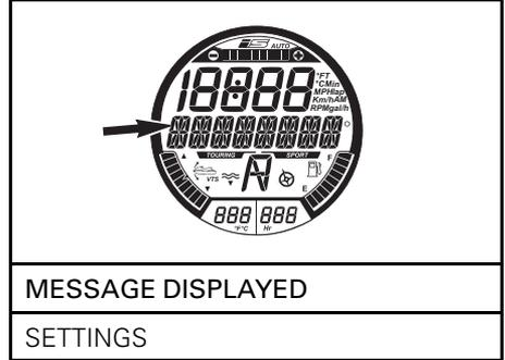
2. Press the UP or DOWN button repeatedly until CLOCK is visible.
