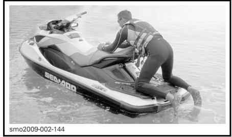
Take hold of the seat strap to help maintain your balance and step forward onto the footboards on either side of the seat.
