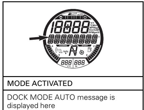
6. Press the UP or DOWN button to toggle the display to DOCK MODE OFF.
