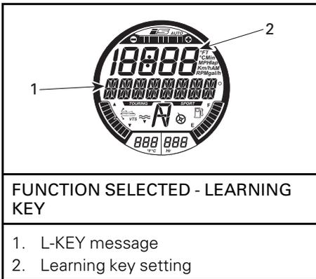
5. Press the UP or DOWN button to toggle the key setting between 1 and 5. See table for speed limitations according to setting.
