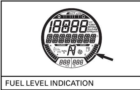
When the fuel tank is full, 8 segments (bars) of the indicator are turned on. The top segment is not used.
