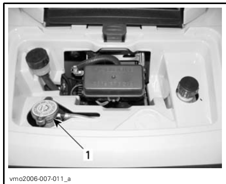
TYPICAL 1. Radiator cap
