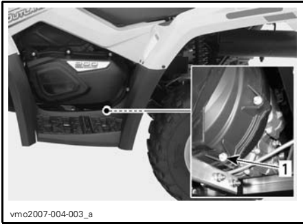
BEHIND LH FOOTREST 1. Drain screw
