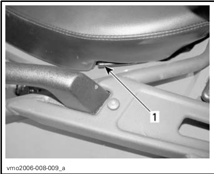
TYPICAL — LH SIDE 1. Seat latch
