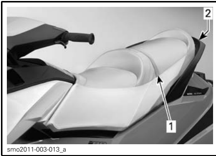
TYPICAL - PASSENGER HANDHOLDS
