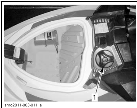
TYPICAL - FUEL TANK CAP LOCATION
