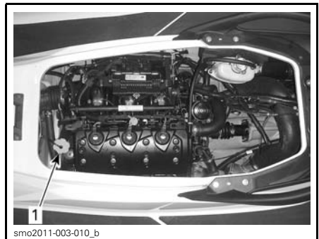
TYPICAL 1. Oil filler cap location
